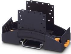
DIN rail housing for use in distribution boards in accordance with DIN 43880, Lower housing part with base latch, width: 35.6 mm, height: 89.7 mm, depth: 48.9 mm, color: black (similar RAL 9005), cross connection: DIN rail connector (optional), number of positions cross connector: 16
