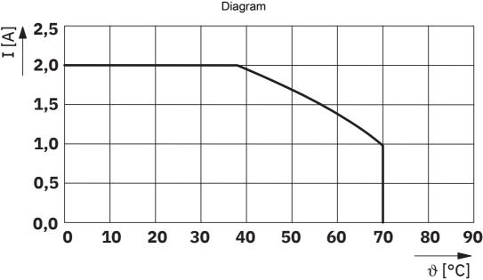
Maximum permissible current per path in uncoiled state
