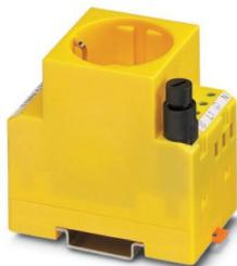
Rail-mountable socket, with glow lamp and equipment fusing 5 x 20 mm to max. 6.3 A; yellow housing
