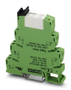
PLC relay, consisting of base terminal block PLC-BSC.../1 IC/ACT with screw connection and pluggable miniature relay, for high inrush currents, for assembly on mounting rail NS 35/7.5, 1 N/O contact, input voltage 24 V DC, max. inrush current up to 130 A
