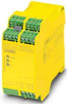
Safety relay for emergency stop and safety door monitoring up to SIL 3 or Cat. 4, PL e in accordance with EN ISO 13849, 1- or 2-channel operation, 3 enabling current paths, nominal input voltage: 24 V AC/DC ... 230 V AC/DC, plug-in screw terminal blocks
