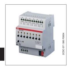
The 8-fold Binary Input BE/S 8.230.1 with manual operation is a rail mounted device for insertion in the distribution board. The device is suitable for reading out 0...265 V AC/DC signals. The inputs are independent of one another.
