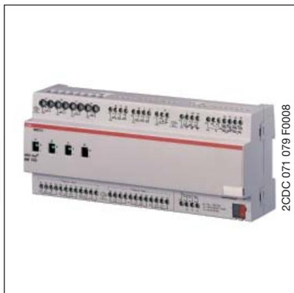
The Room Master Premium is a modular installation device (MDRC) in ProM design. It is intended for installation in the distribution board on 35 mm mounting rails. The assignment of the physical address as well as the parameter settings is carried out with ETS 2 from version V1.3a or higher.
