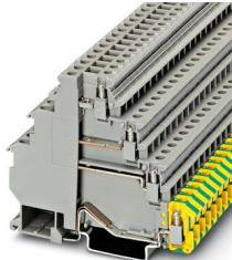
Motor terminal block, four-level, bridgeable, with PE foot, cross section: 0.2 mm<sup>2</sup> - 4 mm<sup>2</sup>, AWG: 24 - 12, connection method: screw connection, width: 6.2 mm, color: gray, mounting type: NS 35/7,5, NS 35/15
