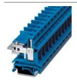
N disconnect terminal block, Special and hybrid connection, Cross section: 2.5 mm² - 25 mm², AWG: 12 - 4, Width: 12.2 mm, Color: blue, Mounting type: NS 35/7,5, NS 35/15, NS 32
