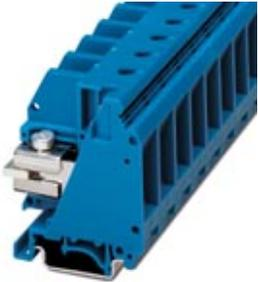
N disconnect terminal block, Special and hybrid connection, Cross section: 0.75 mm<sup>2</sup> - 50 mm<sup>2</sup>, AWG: 18 - 1/0, Width: 15.2 mm, Color: blue, Mounting type: NS 35/7,5, NS 35/15, NS 32
