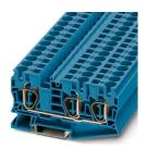
Feed-through terminal block, nom. voltage: 1000 V, nominal current: 57 A, number of connections: 3, connection method: Spring-cage connection, 1 level, Rated cross section: 10  $mm^2$ , cross section: 0.2  $mm^2$  - 16  $mm^2$ , mounting type: NS 35/7,5, NS 35/15, color: blue
