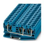
Feed-through terminal block, nom. voltage: 1000 V, nominal current: 76 A, number of connections: 3, connection method: Spring-cage connection, Rated cross section: 16 mm<sup>2</sup>, cross section: 0.2 mm<sup>2</sup> - 25 mm<sup>2</sup>, mounting type: NS 35/15, NS 35/7,5, color: blue
