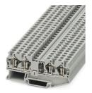
Component terminal block, with integrated diode 1N 5408, nom. voltage: 800 V, nominal current: 1.5 A, number of connections: 4, connection method: Spring-cage connection, Rated cross section: 1 mm², cross section: 0.08 mm² - 6 mm², mounting type: NS 35/7,5, NS 35/15, color: gray
