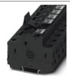
Fuse modular terminal block, Connection method: Screw connection, Cross section: 1.5 mm²- 25 mm², AWG: 16 - 4, Nominal current: 32 A, Nominal voltage: 600 V, Width: 18 mm, Fuse type: Class CC, Fuse type: Glass / ceramics / ..., Mounting type: NS 35/7,5, NS 35/15, Color: black/red
