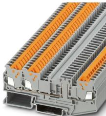
Disconnect terminal block, nom. voltage: 400 V, nominal current: 17.5 A, number of connections: 3, connection method: Quick connection, 1 level, Rated cross section: 1.5 mm<sup>2</sup>, cross section: 0.25 mm<sup>2</sup> - 1.5 mm<sup>2</sup>, mounting type: NS 35/7,5, NS 35/15, color: gray
