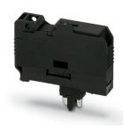
Fuse plug, Prior to replacing the cartridge fuse, disconnect the fuse connector from the basic terminal block., nominal current: 10 A, connection method: Plug-in connection, fuse type:  $G / 6.3 \times 32$ , mounting type: Plug-in mounting, color: black
