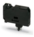
Fuse plug, Prior to replacing the cartridge fuse, disconnect the fuse connector from the basic terminal block., nom. voltage: 630 V, nominal current: 10 A, connection method: Plug-in connection, fuse type: G / 6,3 x 32, mounting type: Plug-in mounting, color: black
