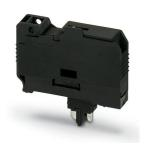
Fuse plug, Prior to replacing the cartridge fuse, disconnect the fuse connector from the basic terminal block., nominal current: 10 A, connection method: Plug-in connection, fuse type: G /  $6.3 \times 32$ , mounting type: Plug-in mounting, color: black
