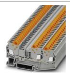
Feed-through terminal block, Connection method: Quick connection, Cross section: 0.5 mm² - 2.5 mm², AWG: 20 - 14, Width: 6.2 mm, Height: 37.8 mm, Color: gray, Mounting type: NS 35/7,5, NS 35/7,5
