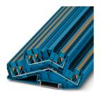
Double-level terminal block, nom. voltage: 800 V, nominal current: 20 A, connection method: Push-in connection, 1st and 2nd level, Rated cross section: 2.5 mm<sup>2</sup>, cross section: 0.14 mm<sup>2</sup> - 4 mm<sup>2</sup>, mounting type: NS 35/7,5, NS 35/15, color: blue
