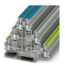
Ground terminal, nom. voltage: 500 V, nominal current: 19 A, connection method: Screw connection, Rated cross section: 2.5 mm<sup>2</sup>, cross section: 0.14 mm<sup>2</sup> - 4 mm<sup>2</sup>, mounting type: NS 35/7,5, NS 35/15, color: gray
