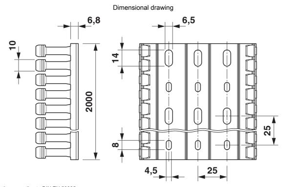
Base perforation according to DIN EN 50085
