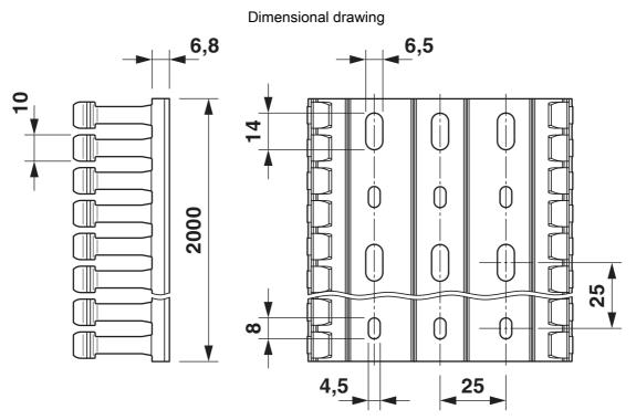
Base perforation according to DIN EN 50085
