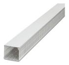
Cable duct for installation and mounting in control cabinets, white, comprising upper part and mounting base, width: 80 mm, height: 80 mm, length: 2000 mm
