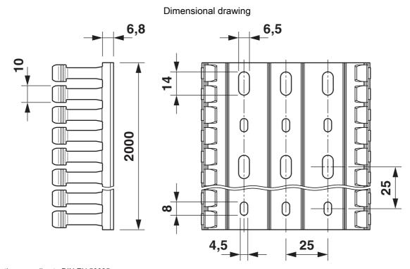
Base perforation according to DIN EN 50085
