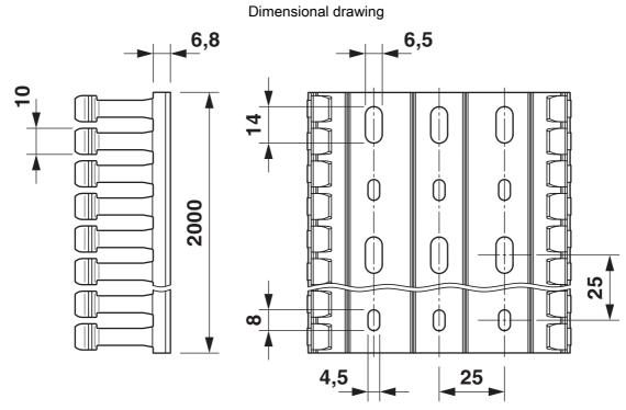
Base perforation according to DIN EN 50085
