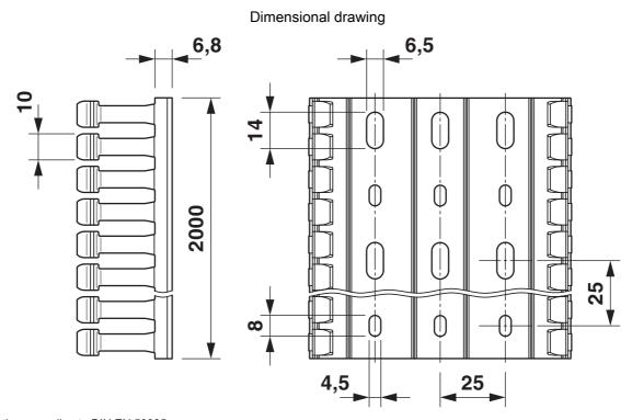
Base perforation according to DIN EN 50085
