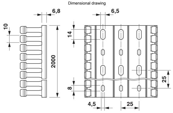
Base perforation according to DIN EN 50085
