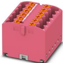
Distribution block, Basic terminal block, nom. voltage: 450 V, nominal current: 24 A, number of connections: 12, connection method: Push-in connection, cross section: 0.14 mm<sup>2</sup> - 4 mm<sup>2</sup>, mounting type: for snapping onto a DIN rail adapter, Direct mounting with flange, Free-hanging, color: pink
