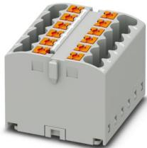
Distribution block, Basic terminal block, nom. voltage: 450 V, nominal current: 24 A, number of connections: 12, connection method: Push-in connection, cross section: 0.14 mm<sup>2</sup> - 4 mm<sup>2</sup>, mounting type: adhesive, color: gray
