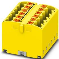
Distribution block, Basic terminal block, nom. voltage: 450 V, nominal current: 24 A, number of connections: 12, connection method: Push-in connection, cross section: 0.14 mm<sup>2</sup> - 4 mm<sup>2</sup>, mounting type: adhesive, color: yellow
