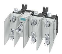
Switch disconnector with fuse in new design lu=250 A, Ue = 690 V, 3-pole for LV HRC fuse Sz. 1 and 2 basic version without 8UC6 handle and shaft
