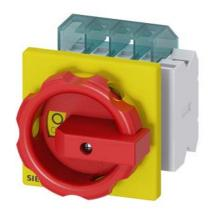
SENTRON, Switch disconnector 3LD, emergency switching-off switch, 3-pole, lu: 16 A, operating power / at AC-23 A 400 V: 7.5 kW, front-mounted, 1 NC, 1 NO, rotary operating mechanism, Red / yellow, 4-hole mounting of the handle
