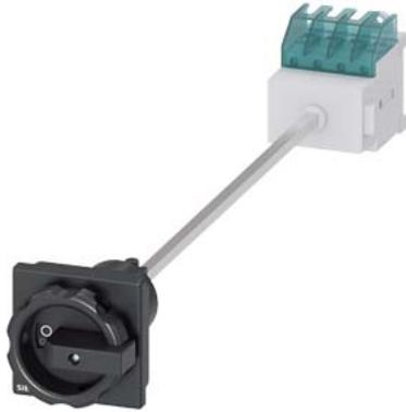
SETRON, Switch disconnecter 3LD, main switch, 3-pole, Iu: 16 A, Operating power / at AC-23 A at 400 V: 7.5 kW, floor mounting with door coupling, rotary operating mechanism, black, 4-hole mounting of the handle
