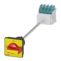
SENTRON, switch disconnector 3LD, EMERGENCY OFF switch, 4-pole, lu: 16 A, Operating power / at AC-23 A at 400 V: 7.5 kW, floor mounting with door coupling, defeatable knob-operated mechanism, red/yellow, 4-hole mounting of the handle
