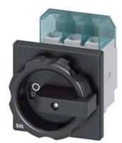
SENTRON, Switch disconnector 3LD, main switch, 3-pole, lu: 25 A, Operating power / at AC-23 A at 400 V: 9.5 kW, front-mounted, rotary operating mechanism, black, 4-hole mounting of the handle
