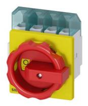
SENTRON, Switch disconnector 3LD, emergency switching-off switch, 4-pole, lu: 25 A, operating power / at AC-23 A 400 V: 9.5 kW, front-mounted, rotary operating mechanism, Red / yellow, 4-hole mounting of the handle
