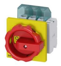
SENTRON, Switch disconnector 3LD, emergency switching-off switch, 3-pole, lu: 25 A, operating power / at AC-23 A 400 V: 9.5 kW, front-mounted, 1 NC, 1 NO, rotary operating mechanism, Red / yellow, 4-hole mounting of the handle
