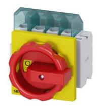
SENTRON, Switch disconnector 3LD, emergency switching-off switch, 4-pole, lu: 25 A, operating power / at AC-23 A 400 V: 9.5 kW, front-mounted, 1 NC, 1 NO, rotary operating mechanism, Red / yellow, 4-hole mounting of the handle
