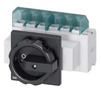
SENTRON, Switch disconnector 3LD, main switch, 6-pole, lu: 25 A, Operating power / at AC-23 A at 400 V: 9.5 kW, front-mounted, 1 NC, 1 NO, rotary operating mechanism, black, 4-hole mounting of the handle
