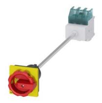
SENTRON, Switch disconnector 3LD, emergency switching-off switch, 3-pole, lu: 25 A, operating power / at AC-23 A 400 V: 9.5 kW, floor mounting with door coupling, rotary operating mechanism, Red / yellow, 4-hole mounting of the handle
