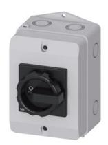
SENTRON, Switch disconnector 3LD, main switch, 3-pole, lu: 25 A, Operating power / at AC-23 A at 400 V: 9.5 kW, molded-plastic encapsulation for metric screw connection, 1 NC, 1 NO, rotary operating mechanism, black
