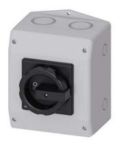
SENTRON, Switch disconnector 3LD, main switch, 6-pole, lu: 25 A, Operating power / at AC-23 A at 400 V: 9.5 kW, molded-plastic encapsulation for metric cable gland, rotary operating mechanism, black
