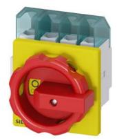
SENTRON, Switch disconnector 3LD, emergency switching-off switch, 4-pole, Iu: 32 A, operating power / at AC-23 A 400 V: 11.5 kW, front-mounted, rotary operating mechanism, Red / yellow, 4-hole mounting of the handle
