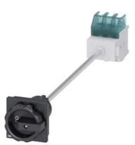
SENTRON, Switch disconnector 3LD, main switch, 3-pole, lu: 32 A, Operating power / at AC-23 A at 400 V: 11.5 kW, floor mounting with door coupling, rotary operating mechanism, black, 4-hole mounting of the handle
