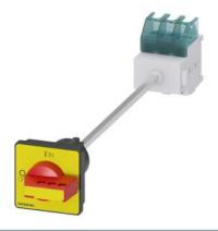
SENTRON, switch disconnector 3LD, EMERGENCY OFF switch, 3-pole, lu: 32 A, Operating power / at AC-23 A at 400 V: 11.5 kW, floor mounting with door coupling, defeatable knob-operated mechanism, red/yellow, 4-hole mounting of the handle
