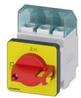
SENTRON, Switch disconnector 3LD, emergency switching-off switch, 3-pole, Iu: 32 A, operating power / at AC-23 A 400 V: 11.5 kW, front-mounted, knob-operated mechanism, red/yellow, 4-hole mounting of the handle
