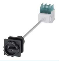
SENTRON, Switch disconnector 3LD, main switch, 3-pole, lu: 32 A, Operating power / at AC-23 A at 400 V: 11.5 kW, floor mounting with door coupling, rotary operating mechanism, black, central mounting 22.5 mm of the handle
