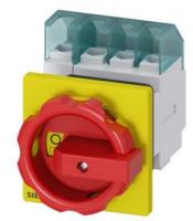
SENTRON, Switch disconnector 3LD, emergency switching-off switch, 4-pole, Iu: 32 A, operating power / at AC-23 A 400 V: 11.5 kW, front-mounted, rotary operating mechanism, Red / yellow, central mounting 22.5 mm of the handle
