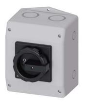
SENTRON, Switch disconnector 3LD, main switch, 6-pole, lu: 32 A, Operating power / at AC-23 A at 400 V: 11.5 kW, molded-plastic encapsulation for metric screw connection, 1 NC, 1 NO, rotary operating mechanism, black
