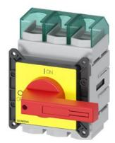
SENTRON, Switch disconnector 3LD, emergency switching-off switch, 3-pole, lu=250 A, operating power / at AC-23 A 400 V: 132 kW, front-mounted, knob-operated mechanism, red/yellow, 4-hole mounting of the handle
