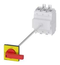
SENTRON, Switch disconnector 3LD, emergency switching-off switch, 3-pole, lu=250 A, operating power / at AC-23 A 400 V: 132 kW, floor mounting with door coupling, knob-operated mechanism, red/yellow, 4-hole mounting of the handle
